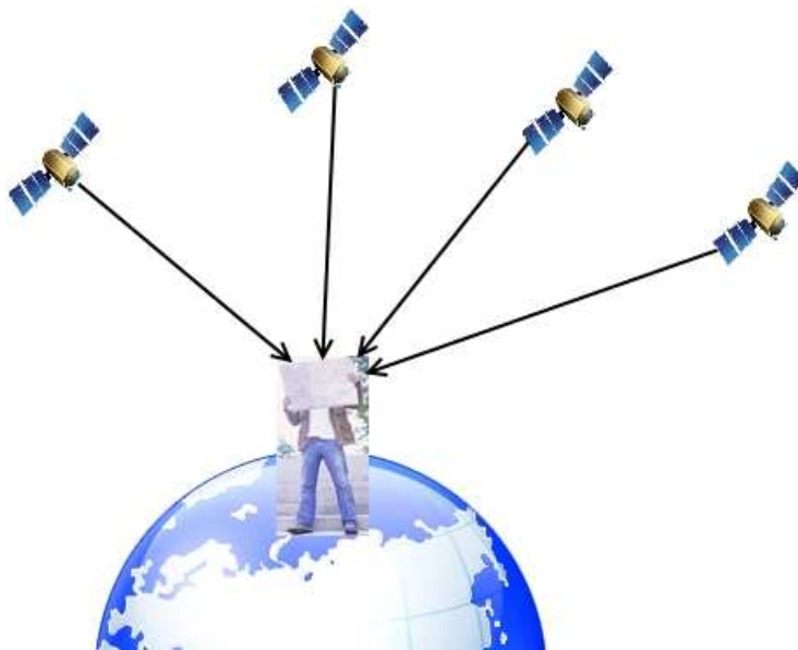
Figure 10. Four satellites are needed for accurate positioning in GPS system.
