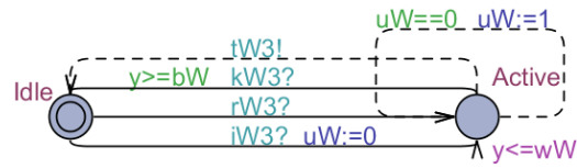
Fig. 26. Automaton core 3,W in the concrete model
