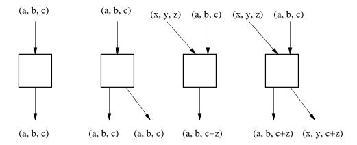
After the last stage of the PREFIX circuit has performed its computation, the records have become  $\{(4, -6, 0), (2, -4, -5), (4, 11, 5), (2, 12, 5), (1, 15, 14), (1, 16, 14), (3, 17, 12), (3, 18, 12)\}$ . Note in particular that  $v_4 = 0$ ,  $v_1 = 14$ ,  $v_2 = 5$ , and  $v_3 = 12$ , as required. The four memory records (4, -6, 0), (2, 12, 5), (1, 16, 14), and (3, 18, 12) now retrace their paths through the MAU to return to their respective memory locations.  $\Box$
