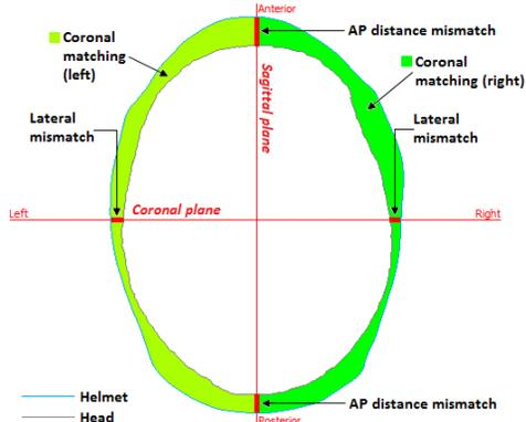
Figure 7. Measures of fit between the helmet and head, as displayed in the Helmet Fit Viewer's viewing panel.
