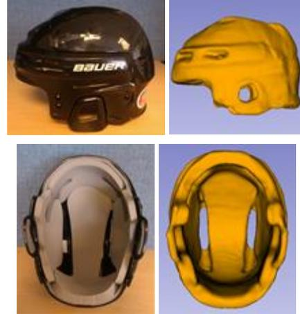
Figure 1. Left: a Bauer 3500 hockey helmet. Right: the 3D model produced by a Kinect scan of this helmet. Top row shows a side view and bottom row shows an interior view.
