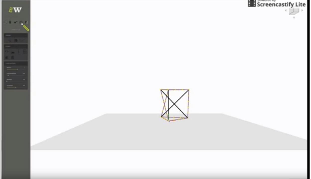
**Figure 18** Stable tensegrity 3-prism created in *PushMePullMe3D*.
