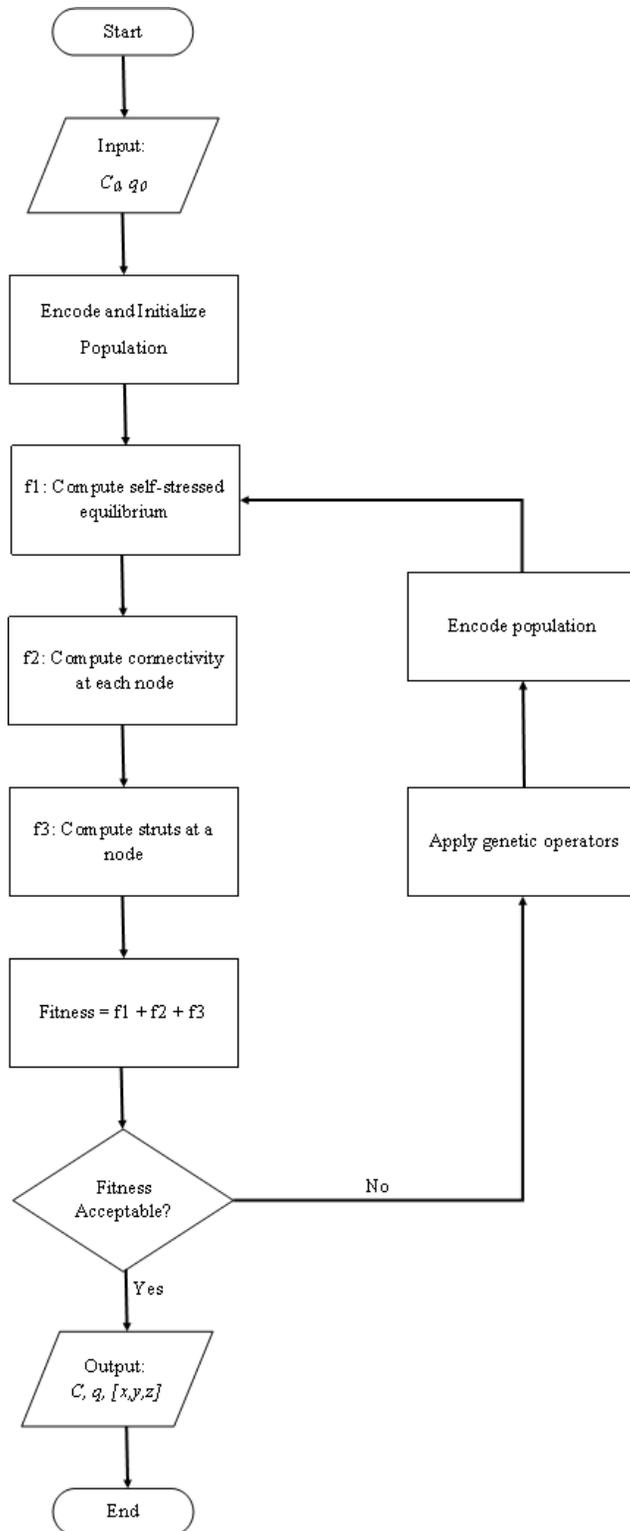
**Figure 14** Flowchart illustrating the workflow used by Yamamoto for tensegrity form-finding using genetic algorithms. Figure by Nuwan Perera based on careful investigation of work by Yamamoto et al [2].
