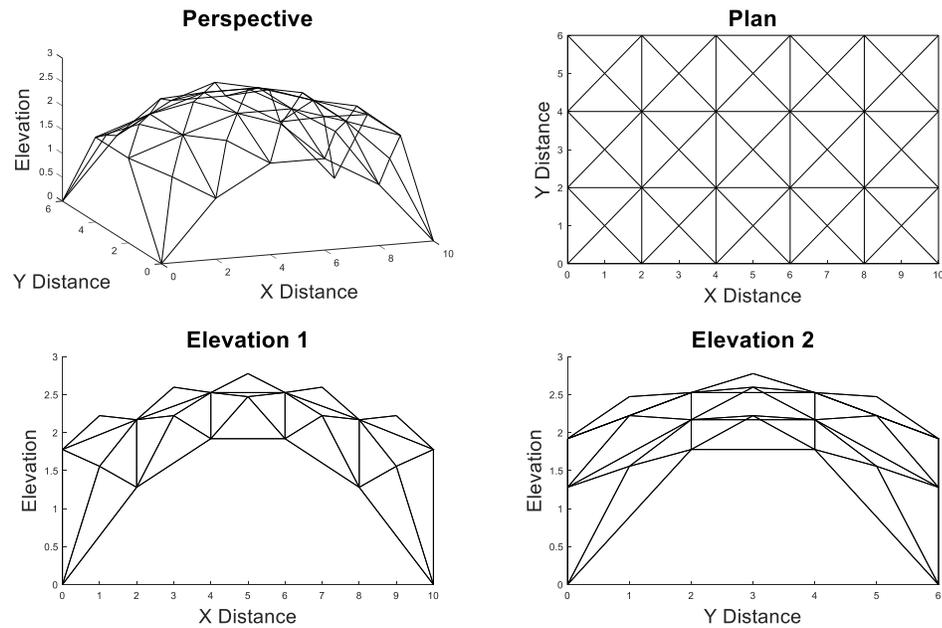
**Figure 8** Sample form-finding of a membrane shell structure using the force density method implemented by the MATLAB code in Fund's thesis. *Perspective*, *Elevation 1*, and *Elevation 2* show different angles of the output shell structure. *Plan* shows the topology graph input of the shell structure. The four corners of the membrane shell structure are fixed nodes anchored to the ground producing an inverted catenary curve. Figure 4-4 from [1]: Reproduced with permission from Ariane Fund.
