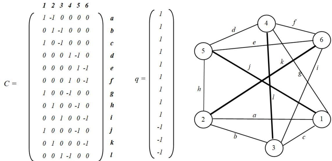
**Figure 11** Connectivity matrix and tension coefficient vector representing a tensegrity 3-prism (right). Figure created by Nuwan Perera adopted from work by Yamamoto et al [2].
