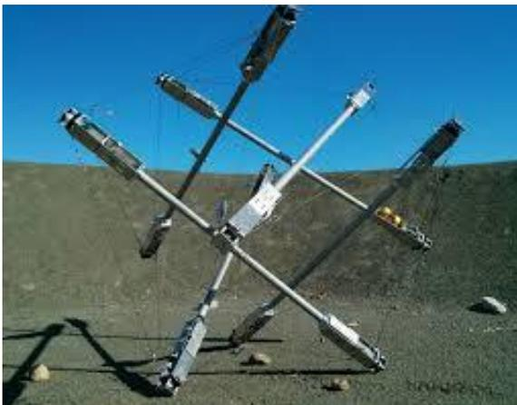
**Figure 7 NASA Superball tensegrity robot.** Image from Wikimedia Commons [20].
