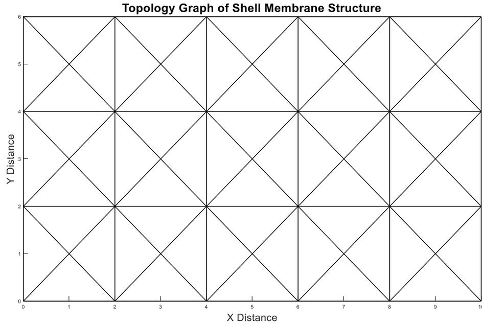
**Figure 9 Planar topology graph used as input for form-finding of membrane shell structures in Fund's thesis.** Reproduced with permission from Ariane Fund [1].
