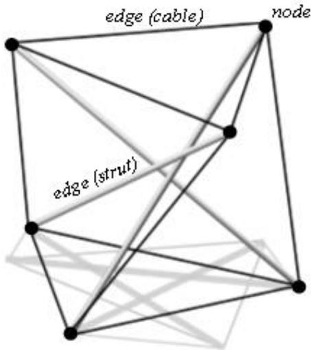
**Figure 3 Representation of a tensegrity structure as a graph showing nodes and edges in 3D.**
