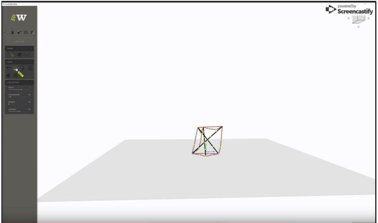
**Figure 19** An unstable 3-prism tensegrity structure collapsing in *PushMePullMe3D*. The buckling of the cables (purple) is shown as the structure collapses.
