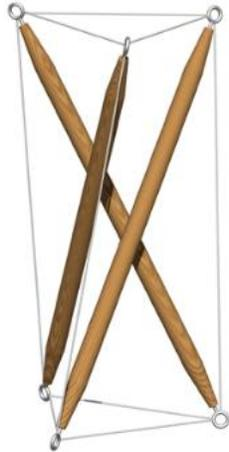
**Figure 1** A 3-strut tensegrity prism showing the connectivity of struts and cables. Image from Wikimedia Commons [3].
