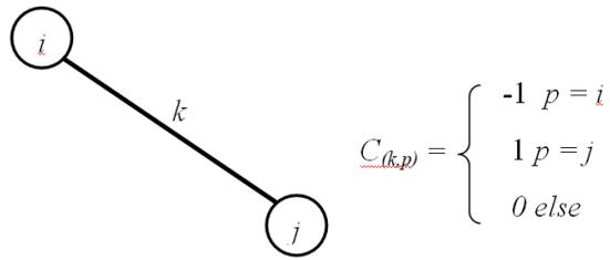
**Figure 10** Example of an edge connected by two nodes and its representation in a connectivity matrix. Figure created by Nuwan Perera adopted by work from Gan et al [31].
