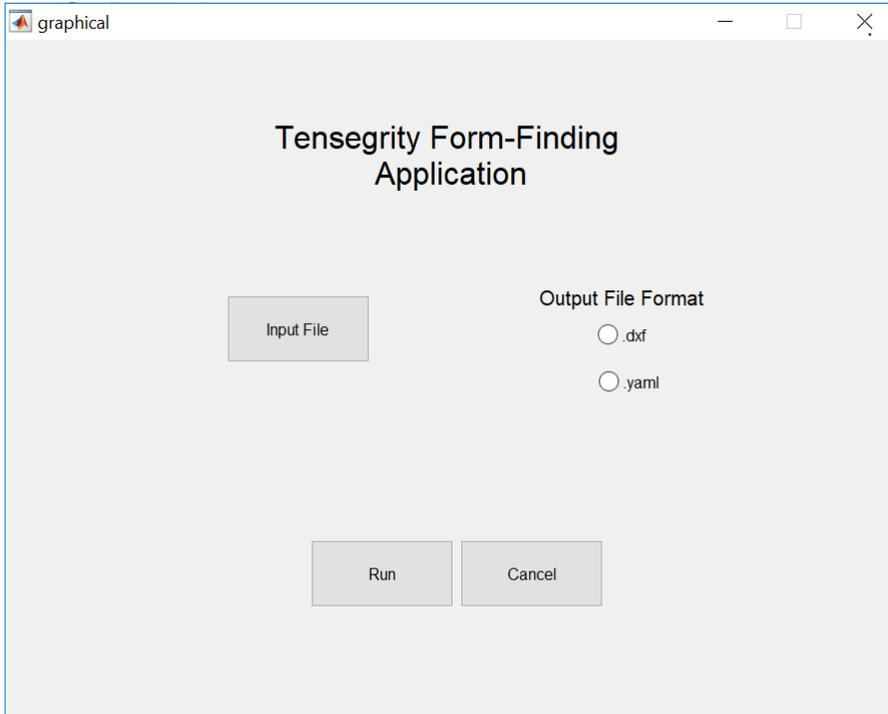
**Figure 15** MATLAB input user interface for our tensegrity form-finding application. Figure by Nuwan Perera.
