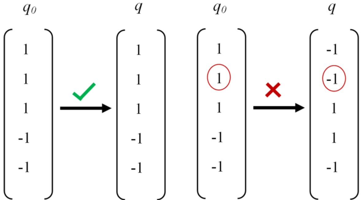
**Figure 16 Resulting force-density vector example. Left: shows a tensegrity structure at self-stressed equilibrium, where the configuration of struts are unchanged. Right: shows an extra strut added and changed configuration indicating a failed tensegrity structure.** Figure by Nuwan Perera.
