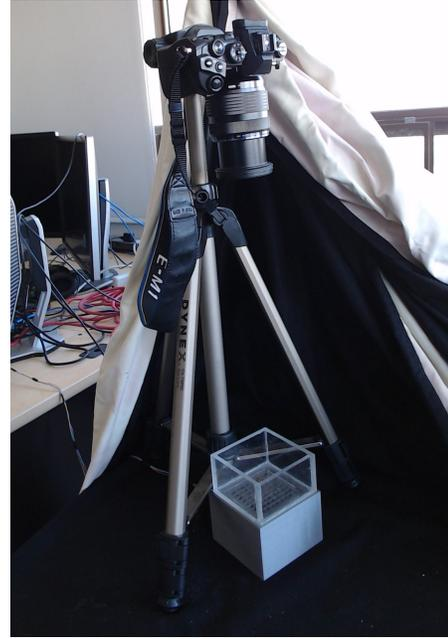
**Figure 2: Multiplexed setup.** A physical construction of Figure 1, where the medium is a milk/water solution at different volumes. The laser array is in the grey box under the container.
