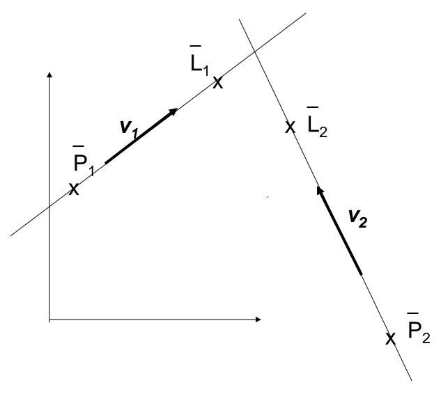
$$\begin{aligned} L_1 &= P_1 + t_1^* \mathbf{V_1} \\ L_2 &= P_2 + t_2^* \mathbf{V_2} \\ &-----\\ L_{1x} &= P_{1x} + t_1^* \mathbf{V_{1x}} \\ L_{1y} &= P_{1y} + t_1^* \mathbf{V_{1y}} \\ L_{1z} &= P_{1z} + t_1^* \mathbf{V_{1z}} \\ \end{aligned}$$
