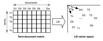
Fig. 1. LSI takes as input a set of documents and the terms occurrences, and returns as output a vector space containing all the terms and all the documents. The similarity between two items (i.e., terms or documents) is given by the angle between their corresponding vectors.
