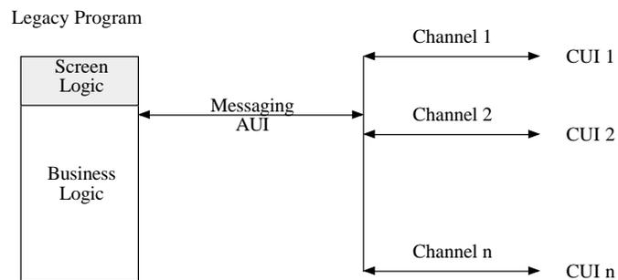
**Fig. 15.** Multi-channel messaging to add plasticity to a legacy system. The user interface is modelled with the AUI and the concrete user interface components communicate through a multi-channel messaging architecture. The concrete user interfaces may be automated teller machines, personal computers, telephones, etc.
