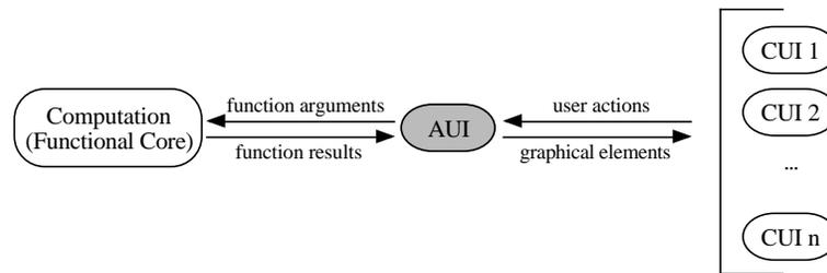
**Fig. 1.** AUI model. A number of concrete user interfaces (CUI's) may be defined for a single AUI. The combination of Computation, AUI and one of the CUI's forms an interactive system.
