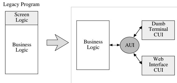
**Fig. 16.** Multi-session architecture for adding plasticity to a legacy system. The AUI models the interface between the user interface logic and the business logic. The AUI also manages the state necessary to achieve multi-session processing.
