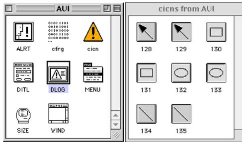
Fig. 12. The Macintosh ResEdit tool was used to define the CUI's visual resources.
