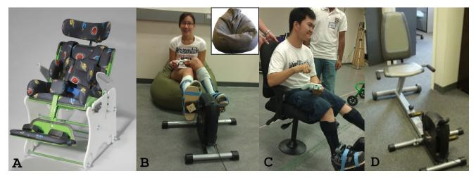
Figure 4. Four chair designs: (A) commercial MSS tilt and recline chair, (B) bean bag chair, (C) modified office chair, and (D) custom designed "racer" chair
