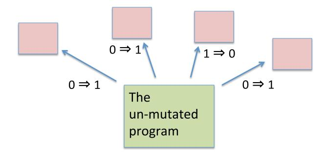
Each arrow represents **one small change**, such as replacing a constant 1 with 0, or exchanging addition for subtraction
