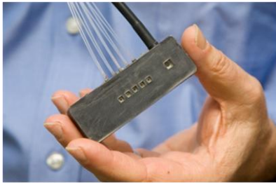
Figure 1. A probe includes a detector (larger square) and four light sources (smaller squares).
