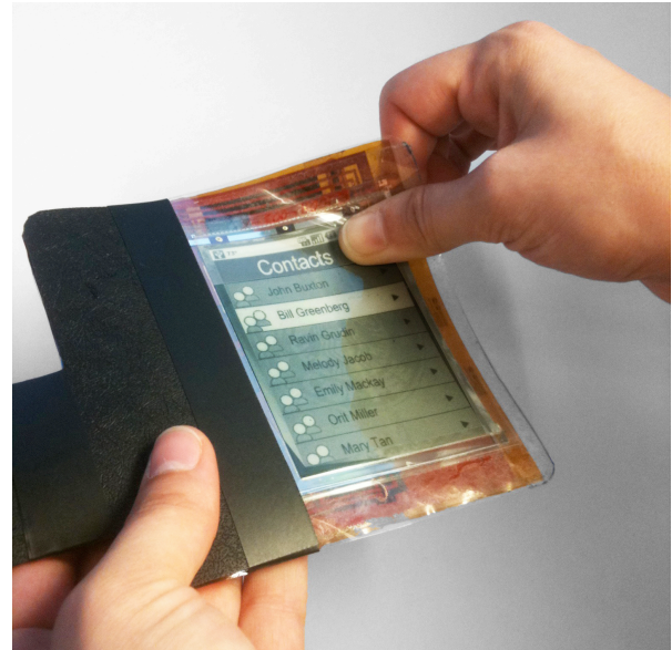
Figure 1. The PaperPhone prototype with flexible E Ink display features bend gesture input recognition.
