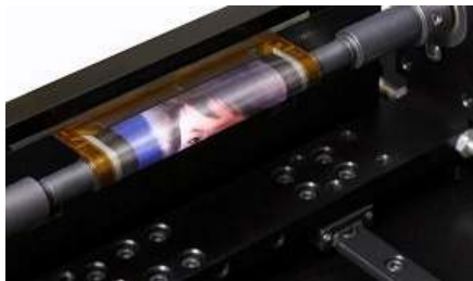
Fig 1. Rollable organic light-emitting diode (OLED) display [9].
