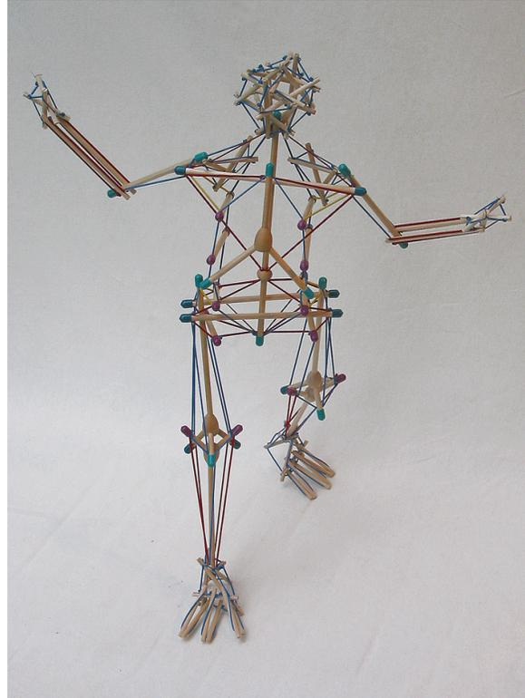
**Figure 14.** Complete tensegrity biped.
