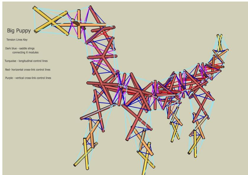
**Figure 6.** Modular tensegrity construction in the Big Puppy. Dark blue: saddle slings connecting X modules. Turquoise: longitudinal control lines. Red: horizontal cross-link control lines. Purple: vertical cross-link control lines. © 2017 Tom Flemons
