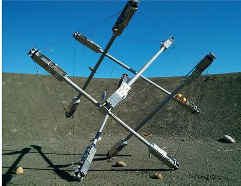
**Figure 11.** The NASA Superball Bot moves using actuators that change cable length. The compliance of the tensegrity structure absorbs landing impact.
