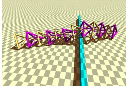
**Figure 12.** Simulation of a tetraspine tensegrity robot crawling over a wall.
