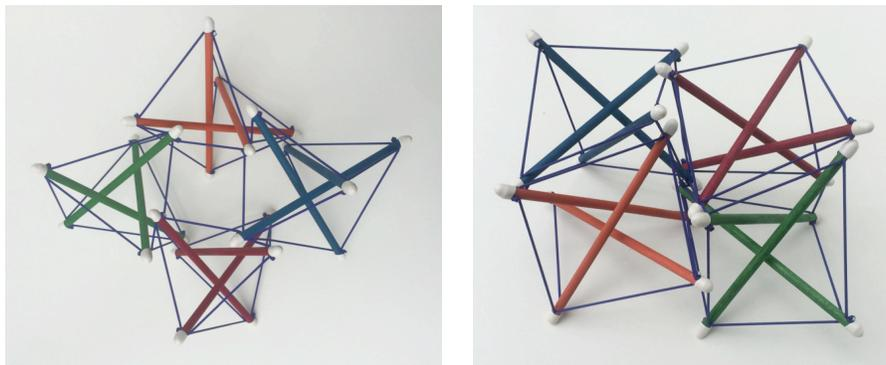
**Figure 7.** A bistable tensegrity-prism hub. The transition between these two stable states is a complex motion with rotation along three axes. © 2017 Tom Flemons
