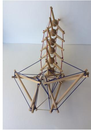
**Figure 5.** Tensegrity pelvis with spine.
