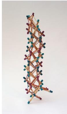
**Figure 1.** Helical tensegrity mast with six control lines creating an 's' curve.
