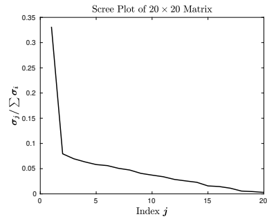
Figure 17.1: Scree plot of a random 20 \times 20 integer-valued matrix. The index k = 2 would be chosen as the rank of approximation of this matrix.
