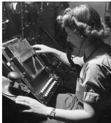
Figure 26.1: A human operated, or interpreted, radar during its early wartime use. Here, a member of the Women's Auxiliary Air Force is observing the radar returns on a cathode ray tube.
