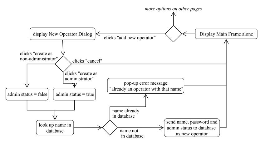
No checking is needed here to make sure the current operator is an administrator. If it is not, these buttons will be disabled or invisible. There was no explicit requirement to check to make sure a new operator was not already in the database, so it's OK if you left this check out of your design.
