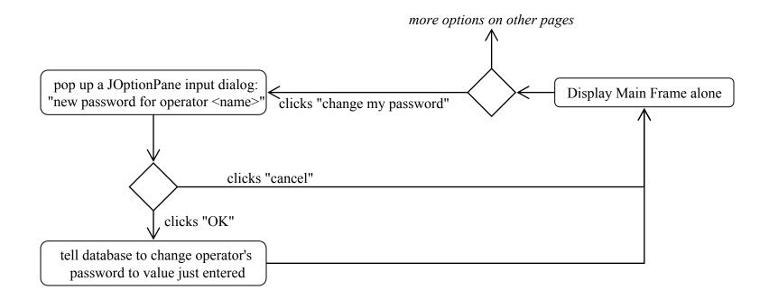
In this section, we're using the operator name that we recorded in Part 1, when the operator logged in. As noted with the log-in dialog picture, ideally we wouldn't echo the password when it is entered. But to keep things simple, it's OK to use a JInputDialog and let it echo the password.
