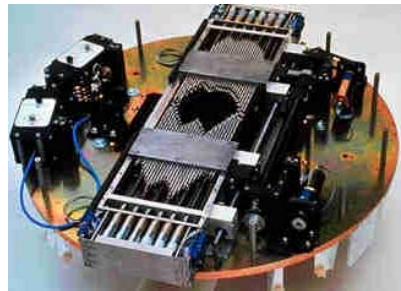
MLC unit, add-on to the LINAC
