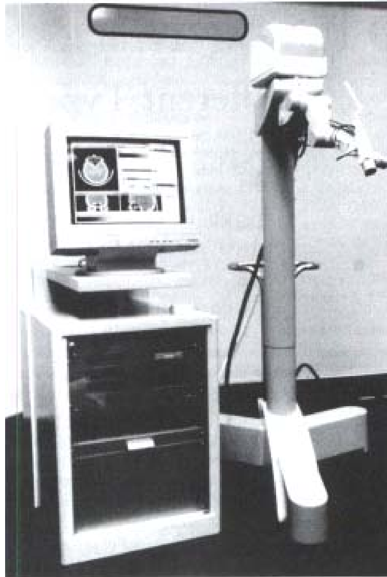
FIGURE 51.2 The Aarhen device for CAS with electro-mechanical measuring arm (coordinate digitizer).
