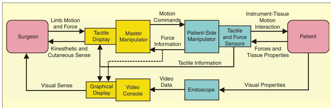
**Figure 3.** The main components of a teleoperated robot for minimally invasive surgery with multimodal haptic feedback. Both force and tactile feedback are included in the model, and graphical display (one method of sensory substitution) is shown as a possible alternative to direct haptic feedback.
