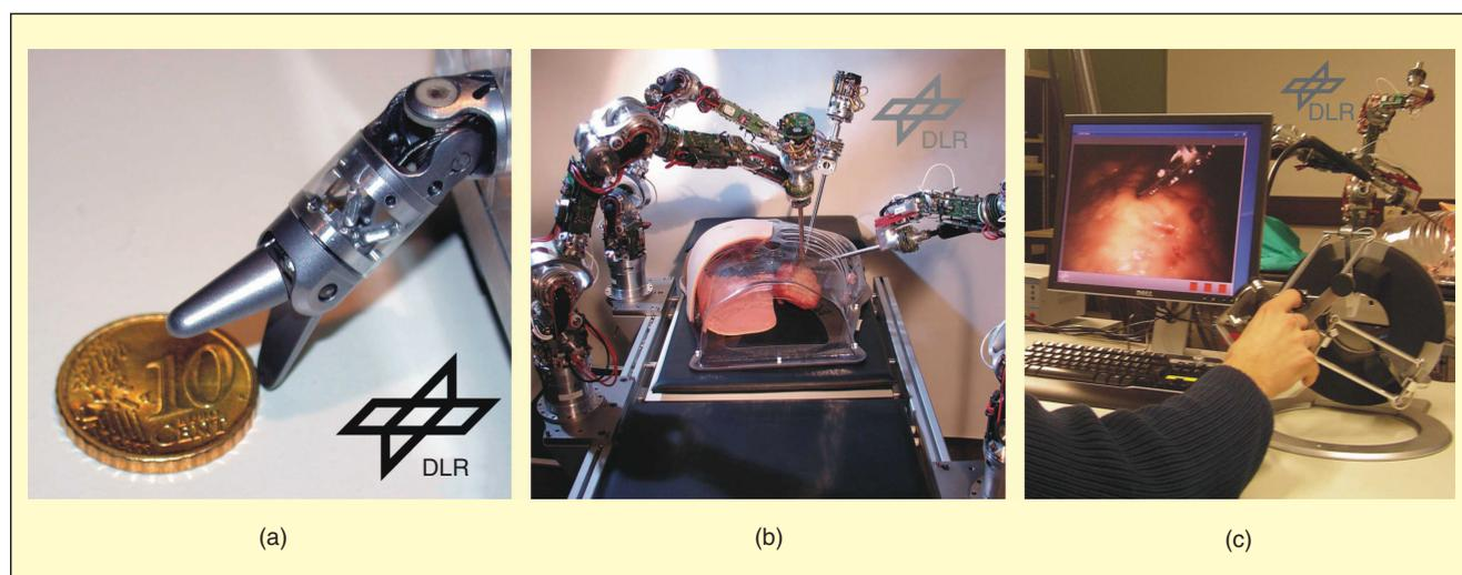
**Figure 4.** A robotic surgery system for two-hand manipulation with integrated force feedback and 3-D vision, designed by researchers at the German Aerospace Centre (DLR), Germany. The system consists of a specially designed dexterous force-sensing instrument, robotic arms and teleoperation controller, and haptic device commercially available from Force Dimension, Inc. (Lausanne, Switzerland) as the master manipulator. Original figures used with permission from B. Kuebler, DLR.
