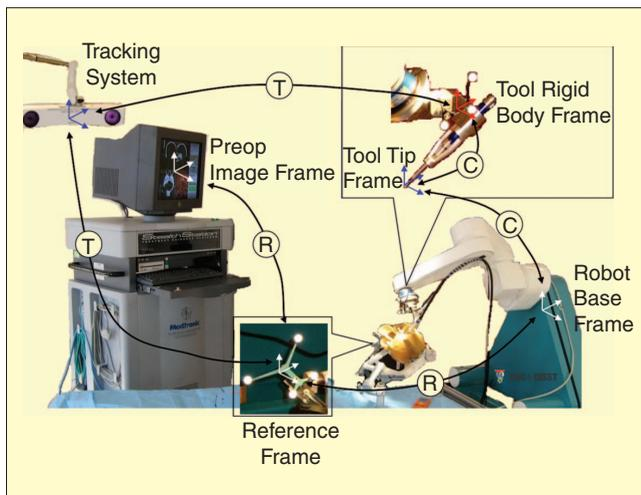
**Figure 5.** Coordinate transformations for a sample image-guided robot system: (T) represents frames that are tracked; (C) represents kinematic calibrations; and (R) represents registration procedures.
