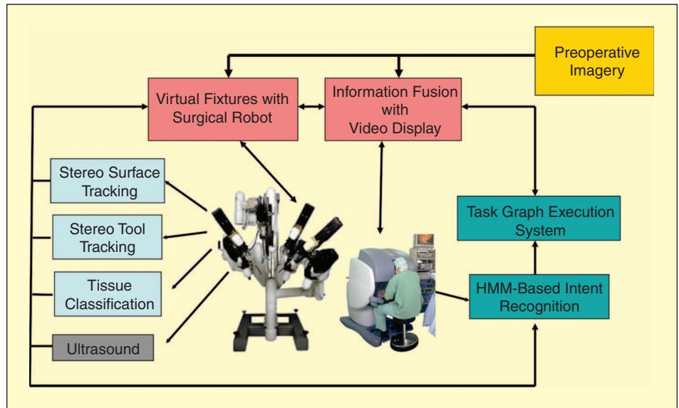
**Figure 1.** The structure of a complete surgical assistant workstation including real-time sensor processing, physical and information augmentation using preoperative imagery, and a task-monitoring system.
