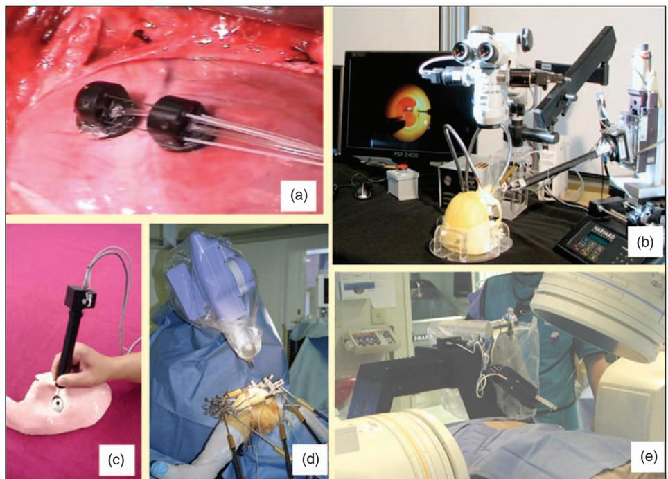
**Figure 2.** Robots for surgical assistants. (a) The Heartlander [37]. (b) The JHU steady-hand robot for retinal surgery. (c) Carnegie Mellon University (CMU) micron. (d) Acrobot for knee surgery. (e) JHU remote center of motion (RCM) robot for nerve and facet blocks in clinical trial at Georgetown University.
