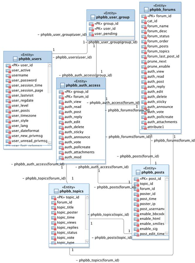
**Fig. 3.** A snippet of the recovered ER data model diagram for PhpBB 2.0
