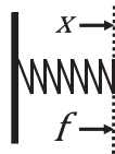
Figure 8.1: A scalar Hookean spring, where x is the displacement and f is the spring force.
