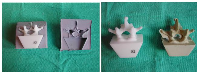
**Figure 3:** Steps in a custom model casting. (1) The two-part mould and the template. (2) The original prototyped model and the final cast model.
