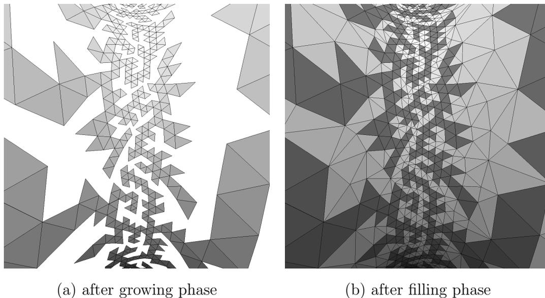
Figure 7: A closeup of the peanut middle after each phase. In (a), no more triangles can be extended into the gap without encroaching too closely to an already-existing triangle. In (b), the light triangles were produced by the filling phase. Note that one triangle pair on the right boundary of the gap has changed due to a diagonal flip which reduces the average aspect ratio.
