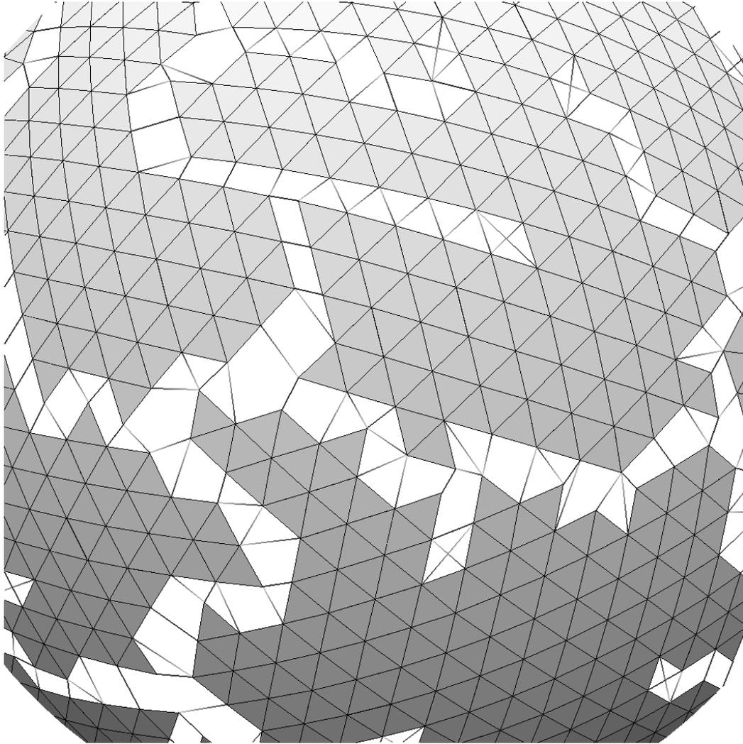
Figure 5: The gap with the closest neighbour relationships on a sphere. The thick uniformly coloured lines between two vertices  $u$  and  $v$  indicate  $u \leftrightarrow v$ . A dark line that fades to a lighter colour from a vertex  $u$  to a vertex  $v$  indicates  $u \rightarrow v$ .
