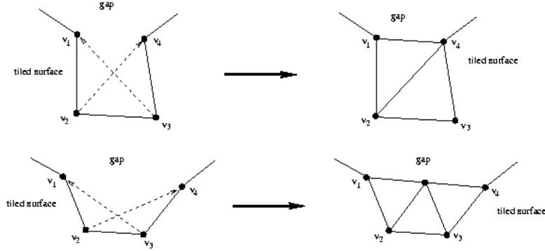
Figure 6: Gap  $X$ 's being filled with and without the addition of another vertex. The nearest neighbour relationships are indicated with dashed lines.
