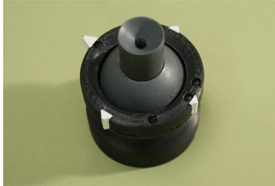
**Fig. 2.** The base of the joystick device. The probe is inserted into the hole on top of the small cylinder and can be tilted with two degrees of freedom. Pressing the probe down to click causes the small cylinder to move into the ball while still permitting the probe to be tilted.
