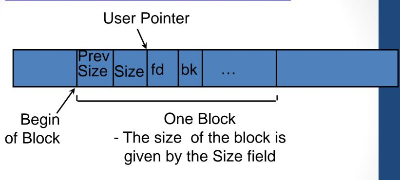
fd (forward) and bk (backward) are only used when the block is unallocated Prev Size and Size are always used
