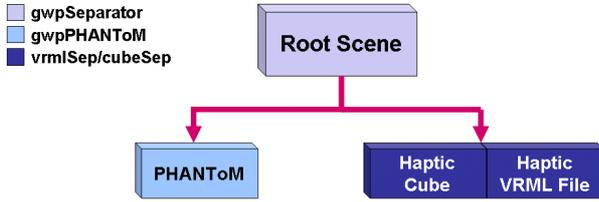
Fig. 5. GHOST SDK scene graph for haptic simulation.
