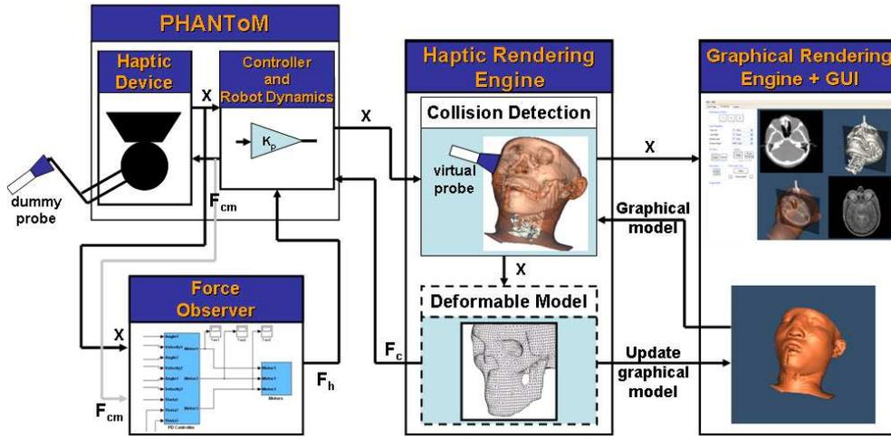
Fig. 2. Proposed system: overall system structure.  $F_c$ : Contact force,  $F_{cm}$ : Force command,  $F_h$ : Hand force,  $X$ : End-effector position.
